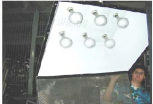
Specifications: Fabricated from a metallic non flammable enclosure. This fixture is used as an overhead softlight. Often this fixture is found with a black fabric drape hung around the bottom so as to direct light straight down.
