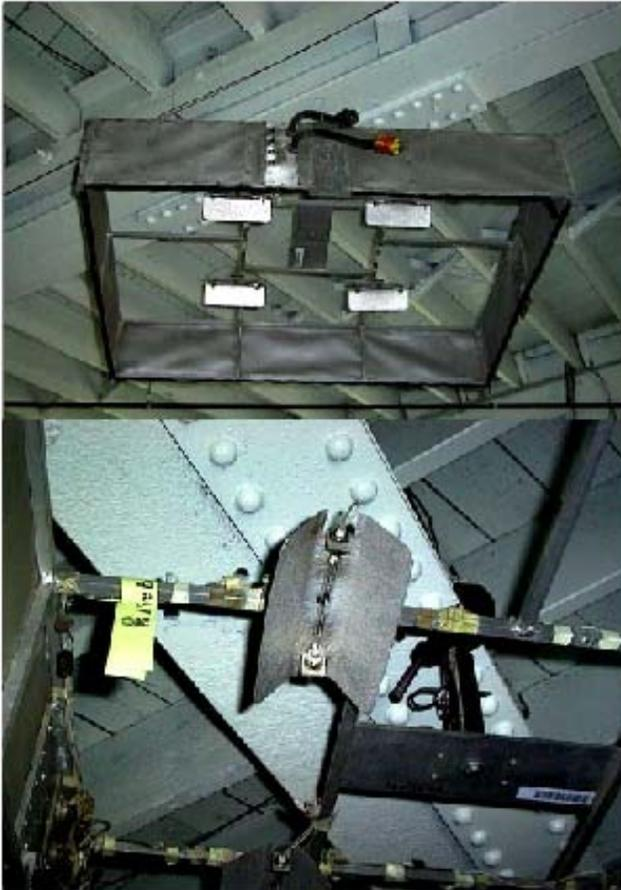
Specifications: Most commonly fabricated from aluminum square tubing. This fixture is used as an overhead soft light. Sides are normally covered with a black shroud so as most of the light is directed straight down through a white drape.
